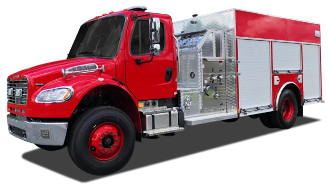
All-aluminum, huck-bolted body designed for long-term durability and maximum storage capacity. This technology provides a lightweight body without sacrificing structural integrity. The design has been verified with stringent Finite Element Analysis (FEA) where the body is stressed to the maximum chassis Gross Vehicle Weight Rating (GVWR) and off-road frame twisting to assure long-term durability.
