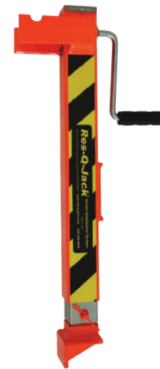
ADD-ON JACK ALX-JACK This jack is made specifically for the Aluminum X-Strut® with a 6,000lbs./2,721kg. lifting capacity and a 2:1 safety factor. Weight: 25lbs./11kg.
