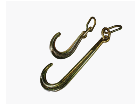
J-HOOKS ACC-JHK8 | 8"/20 cm. ACC-JH15 | 15"/38 cm. These large hooks can attach to a wide variety of structures including posts, axles, or frame components. The hooks are grade 70, rated for 4,700lbs./2,136kg., and come in two useful sizes.
