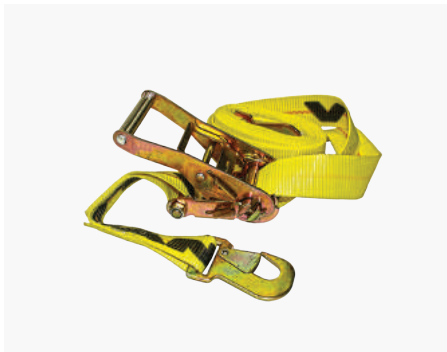
RATCHET STRAP W/ SNAP HOOKS ACC-RSSN This 2"/5cm. x 15'4.5m. medium duty ratchet strap has a WLL of 2,000lbs./909kg., and the snap hooks at each end can hook inside items such as a link of 3/8"/1cm. chain.
