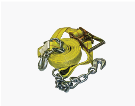
RATCHET STRAP W/ CHAIN ACC-RSCH This 27'/8m. strap is 2"/5cm. wide with a 3,300lbs./1,500kg. WLL. Its attached D-Ring, 3/8"/1cm. chain, and grab hook provide a strong base restraint.
