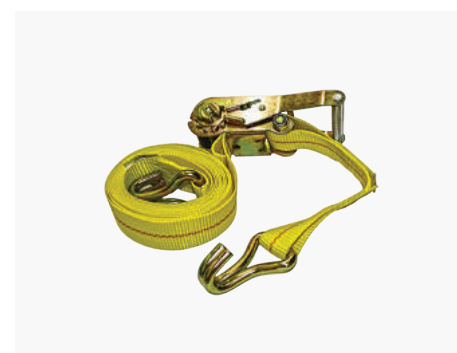
RATCHET STRAP W/ WIRE HOOKS ACC-RSWH This 15'4.5m. strap is 2"/5cm. wide with a 3,300lbs./1,500kg. WLL. It includes ratchet and attached wire hooks which are compatible with our base plates.
