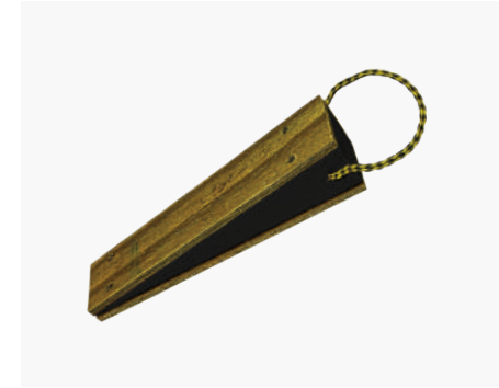
HYBRID WEDGE ACC-WDGE This wedge is made with plastic sandwiched between two pressure treated wood skins, reducing slippage associated with all-plastic cribbing.
